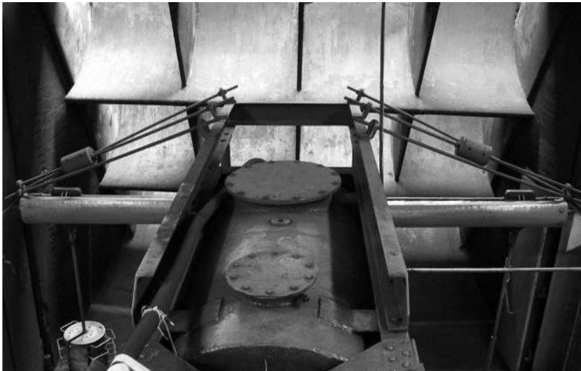
Fig. 5.2. Test stand. The view of the measurement system to measure torque, and air guide
