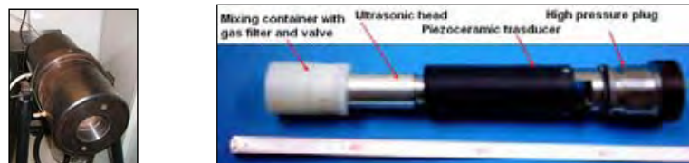
Fig. 6. USHP insert piece made up of four main parts
