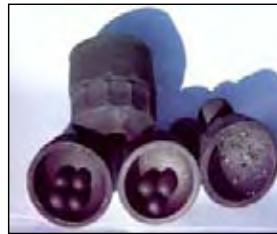
Fig. 4. SiC containers and SiC grinding balls
