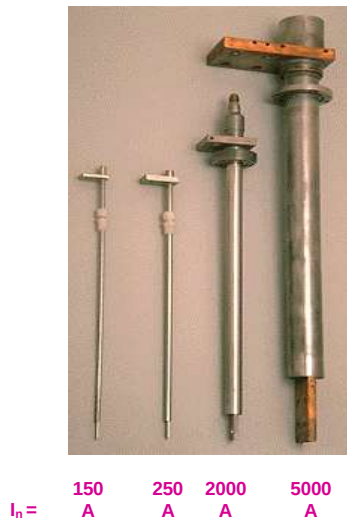
Fig. 5. Conventional current leads
