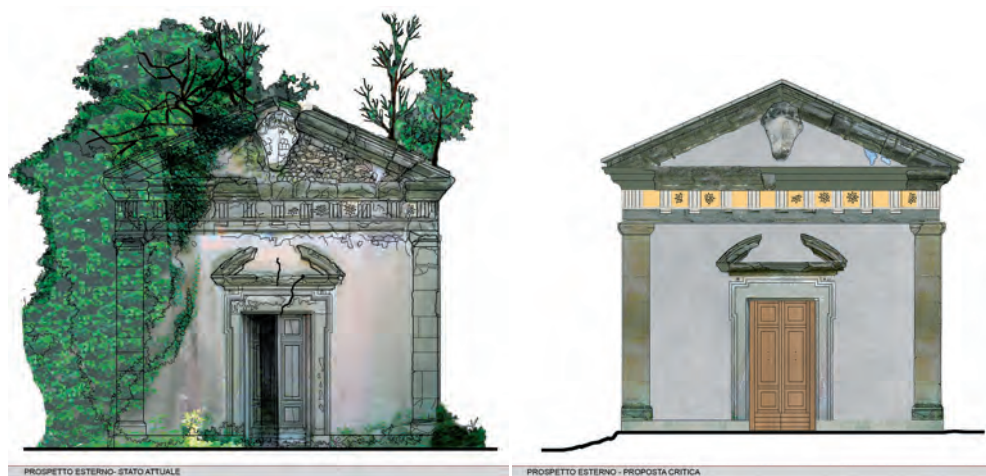
Fig. 5. Restoration of the façade of the chapel in Villa Versaglia at Formello (Rome) (exam project in the Conservation Laboratory, by Caterina Loprencipe, Matteo Mancini, Riccardo Pagani).
