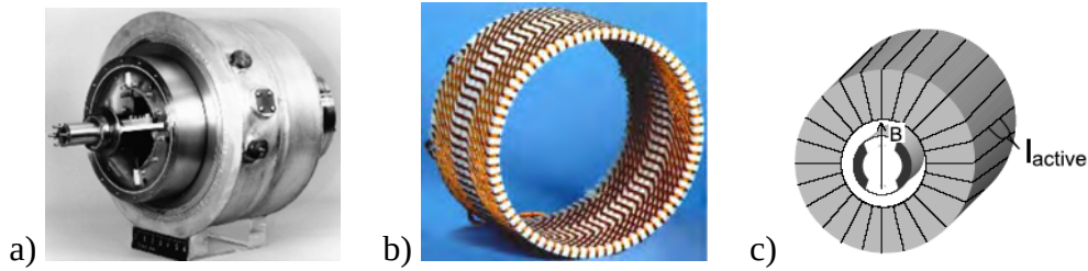
Fig.3 Megawatt generator tested in liquid hydrogen at 20 K, a) generator with high purity aluminium field windings b) copper Litz wire armature with an active length of 4.1 cm, c) Gramme ring armature windings, shown with a short active length. The outer return path of the Gramme ring does not contribute much to power generation or ac loss because B is significantly diminished in this region. The projected frequency is 200-1000 Hz, field 2 tesla.
