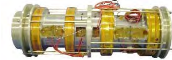
Fig.22 An example of the existing double ADR magnet consists of two sets of coils, each producing 3.0 T. The coils are actively shielded to allow independent operation, and to reduce the stray field. Because the magnet will operate in space, it is completely cryogen-free, and cooled by conduction to a cryocooler. To minimise the heat load to the cooler, the magnet has been wound with ultra-fine superconducting wire (0.1 mm diameter insulated), giving an operating current of less than 2.3 A at full field. [54, http://www.spacecryo.com ].
