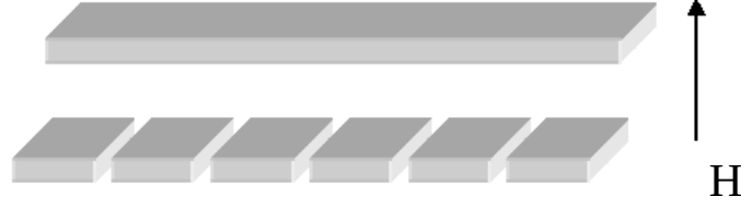
Fig.15 Schematic of the fragment of the single filament and multifilamentary coating in external magnetic field.
