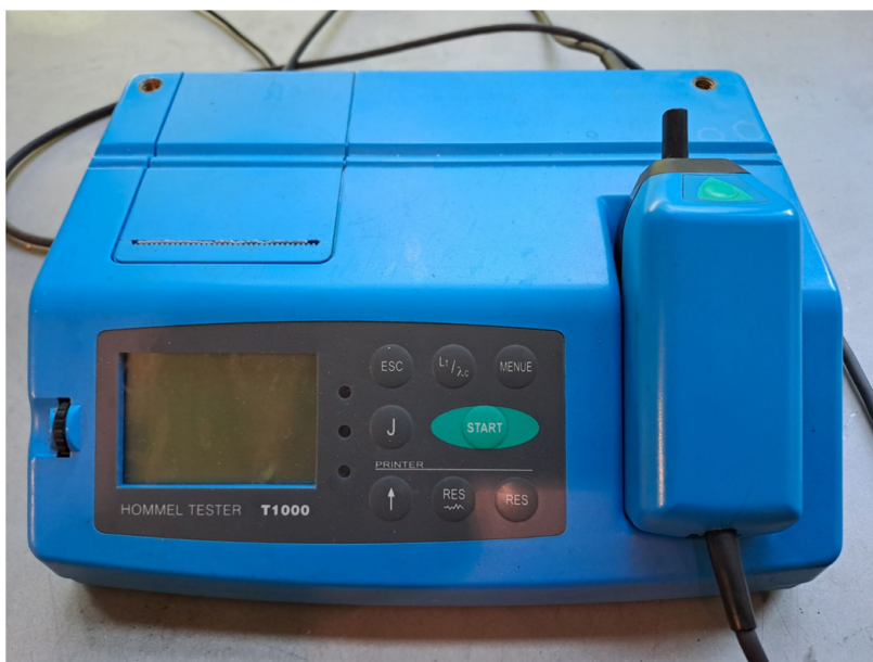
Ryc. 4.3. Profilometr Hommel Roughness Tester T1000
