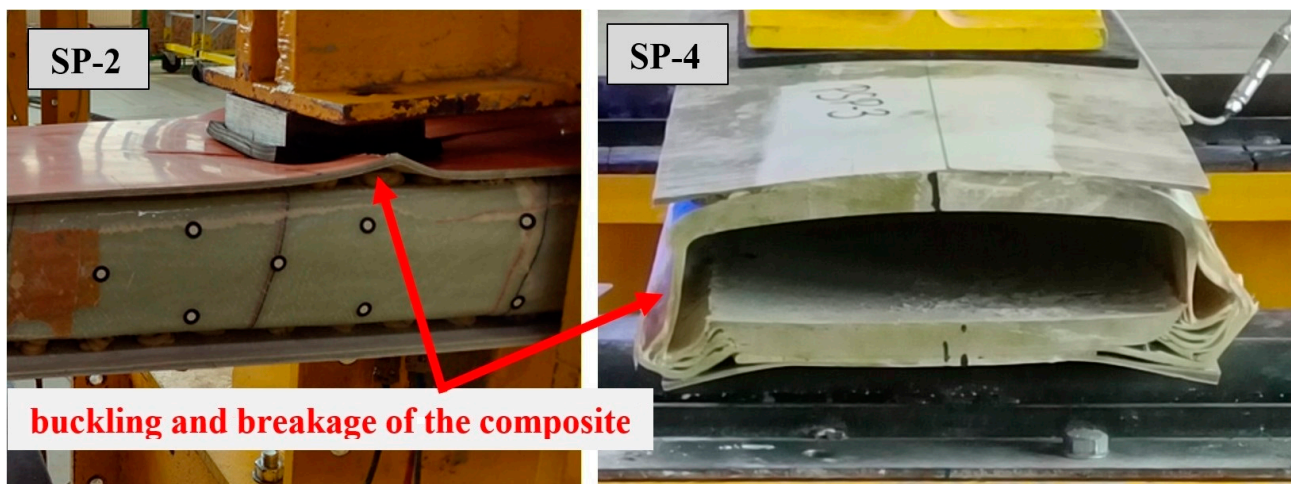
Figure 21. Failure mechanism of the empty closed profiles.
