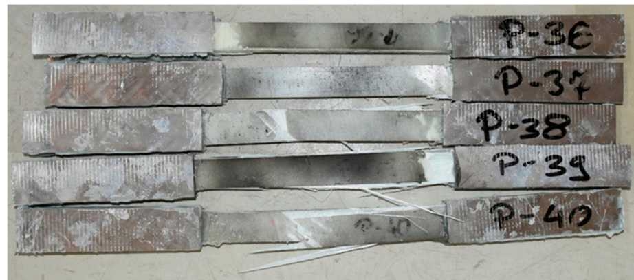
Figure 8. View of Vestas-type blade samples after destruction.
