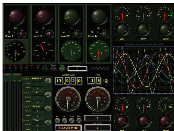
Fig. 3. Developed TGAs subsystem for control of gas flow and electrical parameters.
