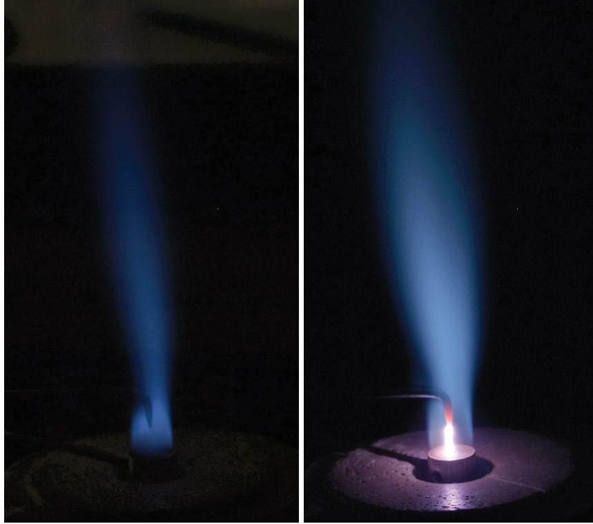
Fig. 5. Photographs of the \text{CH}_4 -air premixed flame without and with TS discharge at \Phi=0.7 (stability limit without discharge) and gas flow rate Q=4 \text{ Nm}^3/\text{h} , photo exposure time 2s, ISO 100, f 5.6.
