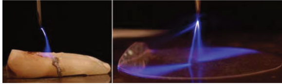
Fig. 2. The oscilloscopic record of positive streamer current pulse ( U = 11.6 kV, f = 11.4 kHz, I_{\max} = 23 mA) and the related photos on teeth and plastic surfaces.
