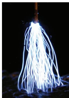
Fig. 2. Photograph of the transient spark with electro-spray of water in 1 cm needle-mesh gap, water flow rate 0.5 mL/min, 14 kV.
