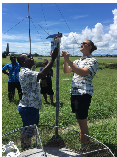
Ryc. 14. Knowing Our Ambient Local Air-quality (KOALA) , tani monitor opracowany przez International Laboratory for Air Quality and Health (ILAQH), Queensland University of Technology w 2018 r.
