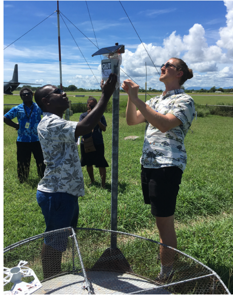
Fig. 14. Knowing Our Ambient Local Air-quality (KOALA), low-cost sensor developed by the International Laboratory for Air Quality and Health (ILAQH), Queensland University of Technology in 2018
