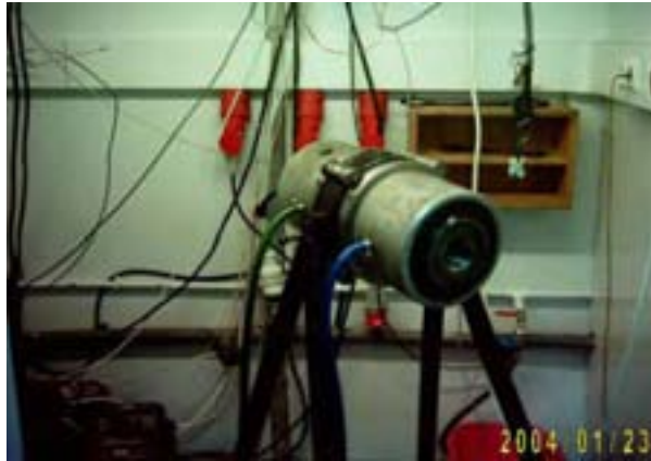
Fig.3. High gas pressure chamber for HIP-ing at pressure up to 1.5 GPa
