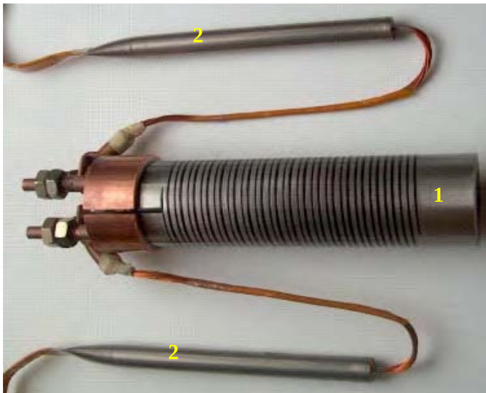
Fig. 1. Superconducting elements of resistive SFCL: 1 – Bi-2212 bifilar coil - C02-034 (NEXANS), 2 – Bi-2223 current leads - CSL-120-L (CAN Superconductors)[5]
