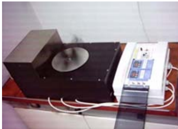
Fig. 4. Three axial rotated ball mill for nanopowder dopant milling
