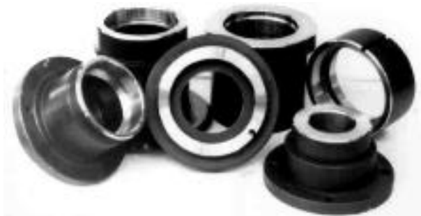
Fig. 3.16. The parts that are subjected to centrifugal cladding by eutectic coating to their internal surface
