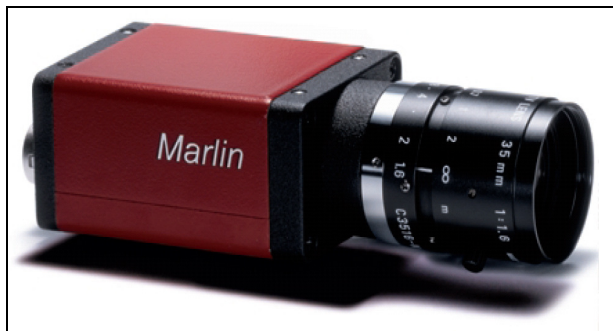
Fig. 17 Used camera AVT Marlin F-033C [61]
