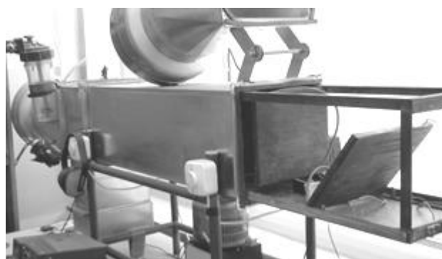
Fig. 2. Filter chamber equipped with cassette with bifilar windings
