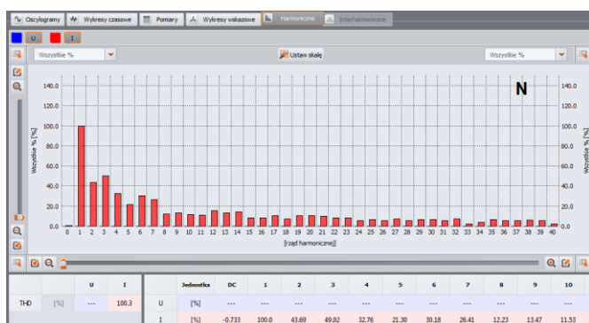
Fig.3. The harmonics current on the power reactor
