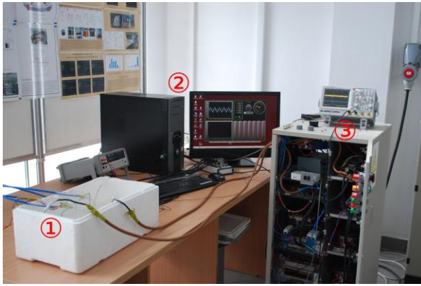
Fig.2. Test stand for measuring the overcurrent response of the tape: 1 – HTS 2G tape in LN 2 bath, 2 – data acquisition, 3 – computer controlled supplying system
