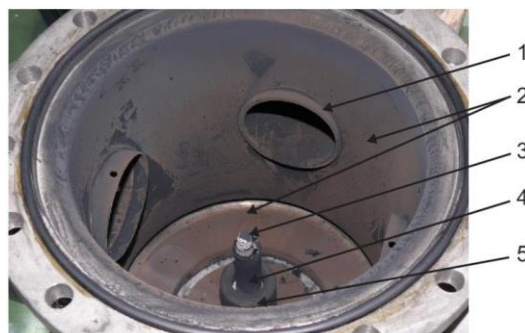
Fig. 1: View inside reactor where: 1- diagnostic window, 2 – carbon elements on reactor walls, 3 – cathode deposit, 4 – cathode, 5 – cathode holder
