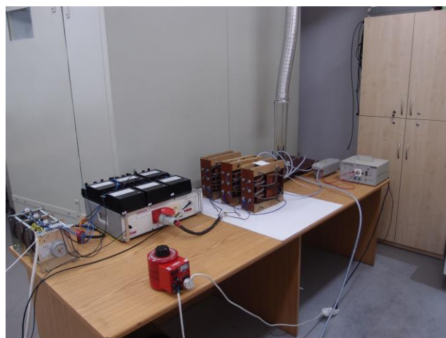
Fig.2. Measuring system of voltage conducted disturbances of plasma reactor type GlidArc
