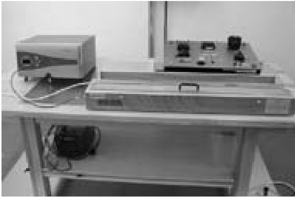
Fig.2. Measuring position with capacitive coupling clamp
