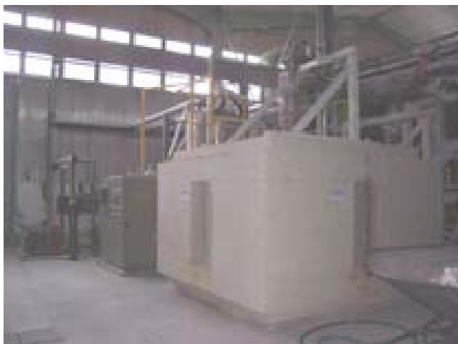
Fig.3. General view of the complete system of the matrix magnetic separator plant for kaolin purification, working in Kaznejov (Czech Republic).
