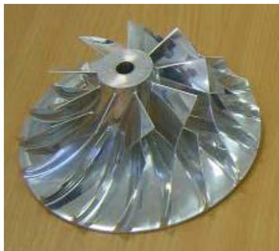
Fig. 2. Liquefier compressor wheel of diameter 250 mm.
