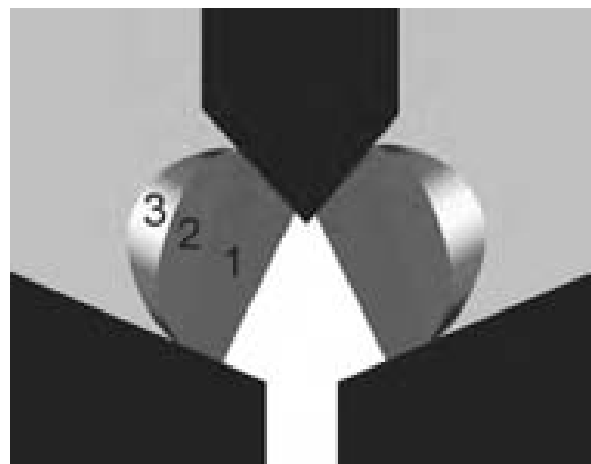
Fig. 3. Draft illustrating the phenomenon of shunting of arc current by the current conducting melt (1 - arc, 2 - gas layer, 3 - layer about consistency liquid - solid shunting arc).
