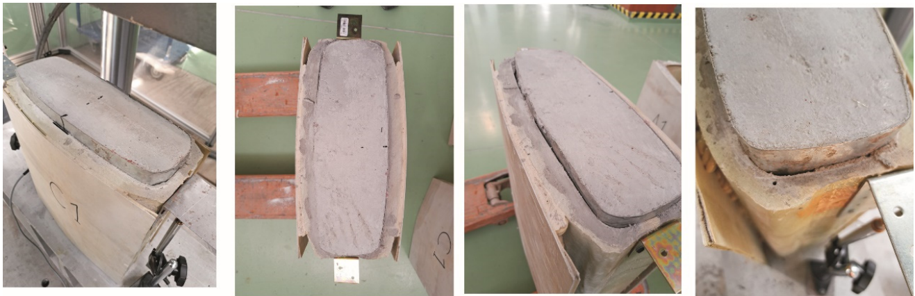
Figure 11. Post-testing push-out specimens.
