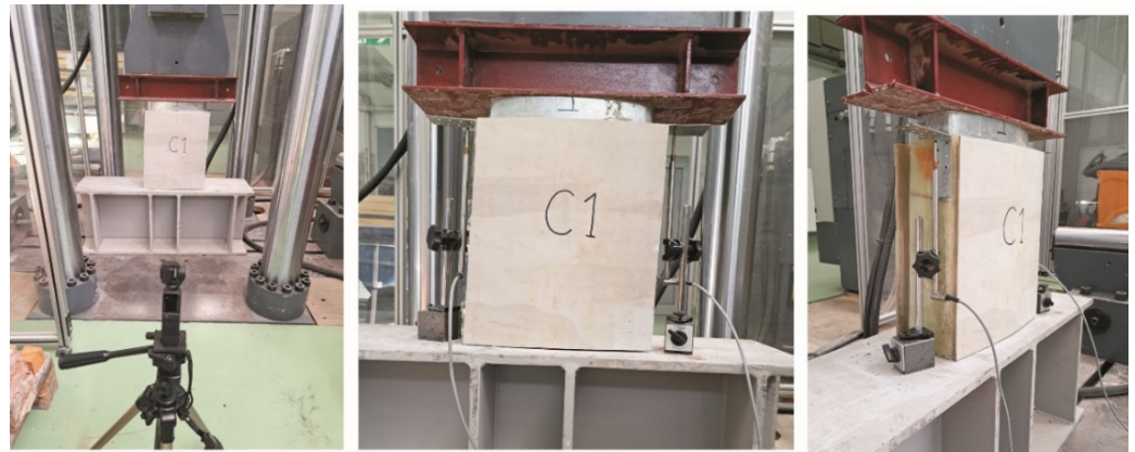
Figure 6. Execution of push-off test.
