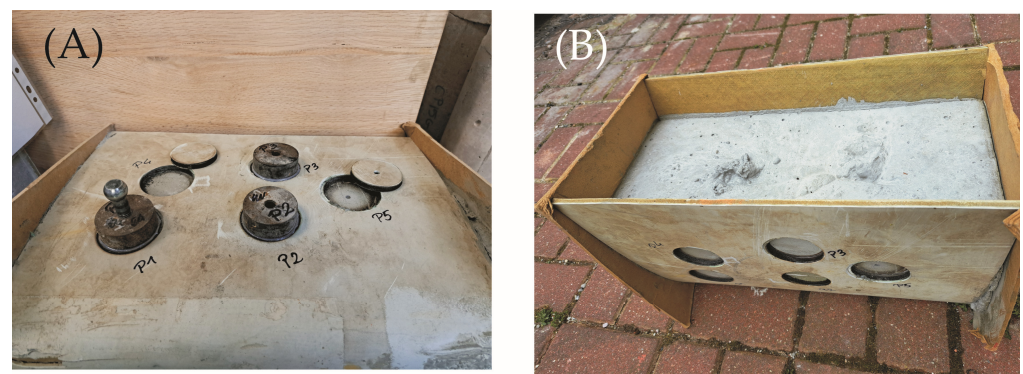
Figure 7. Pull-off test: (A) execution; (B) the specimen after testing.
