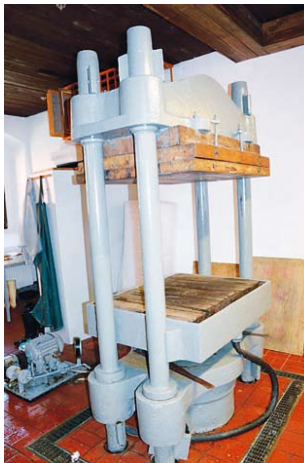
Fig. 55. Paper laying equipment – the press. Photo by A. Fortuna-Marek
