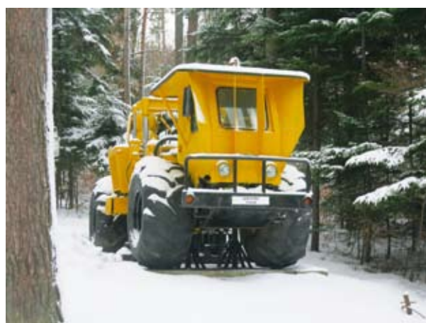
Fig. 58 Vehicle used for raising seismic vibration. Photo by A. Siwek
