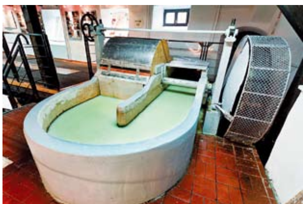
Fig. 54. Paper laying equipment – the 'Hollander Beater'. Photo by A. Fortuna-Marek
