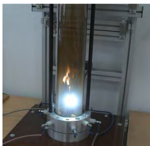
Fig.1. Quasi-arc discharge in plasma reactor, Laboratory of Institute of Electrical Engineering and Electrotechnologies
