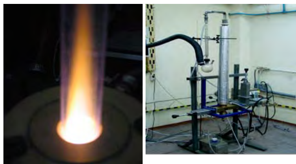
Fig. 1. The microwave plasma – left and the setup for synthesis of carbon nanotubes- right [2]
