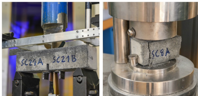
Fig. 1. Illustration of the test configuration used for the fracture testing of specimens in three-point bending (left), and for the subsequent compressive test (right); span was 140 mm.
