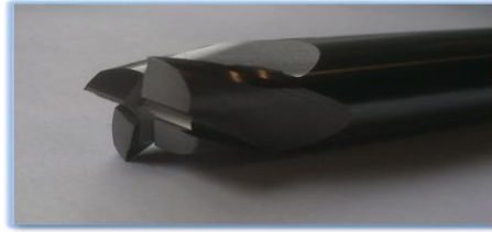
Fig. 3. Slotting mill – used to milling single junction clamps
