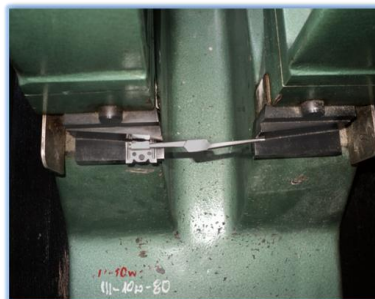
Fig. 8. The placement of a sample in a bearing
